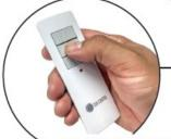
When shade is in the desired position, press and hold the STOP button to set the top limit position. The motor will motor make a brief movement (jogs) in both directions
